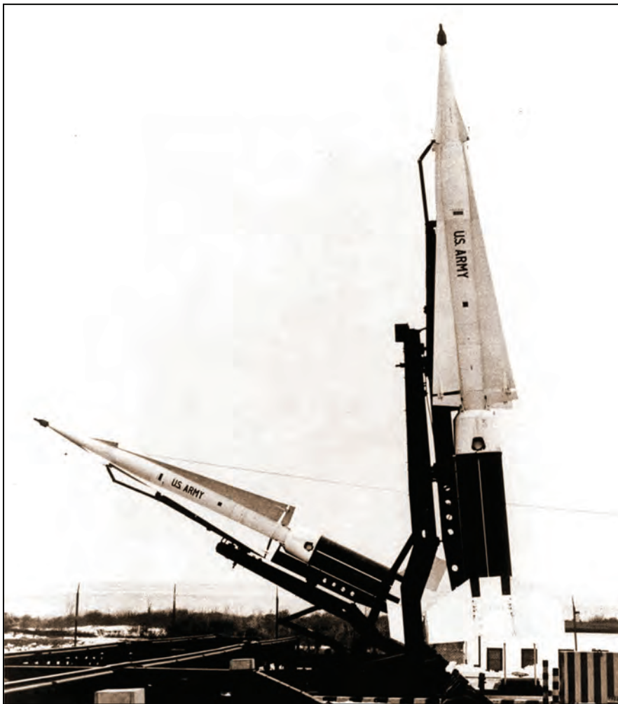
Typical Hercules Missiles as seen at Ft. Hancock base at Sandy Hook. The missile at right is in upright firing position on its launcher, while the other missile is only partly raised. Each missile was 41 feet long with its booster, 31.5-inches in diameter, 6-foot wingspan, and weighed of over 10,000 pounds. 56
